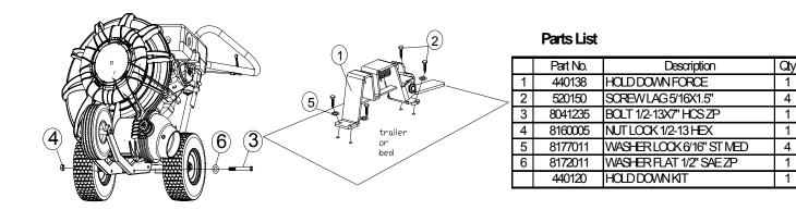
To use the Hold Down, simply rest the bolt mounted previously behind the tire in the slot area that the pin will retract. Using your foot press the lever and lower the blower into the Hold Down unit gently unit it rests at the bottom of the slot. To release simply reverse order used to Hold Down unit.
